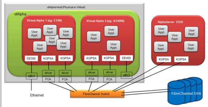
The vtAlpha host computer gets equipped with FibreChannel adapters (FCA) that connect to the FibreChannel based company storage fabric. vtAlpha includes the software drivers for these FCA's, this was included in v2.3.
